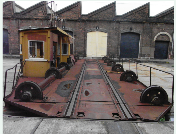
The only remaining in-situ 'traverse' at Eveleigh, used to transport carriages between tracks. Photo - Graham Quint
